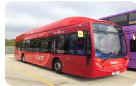
Compressed biomethane stored on roof
